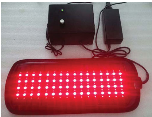
Figure 4. The assembly of the red and infrared LED phototherapy device.
